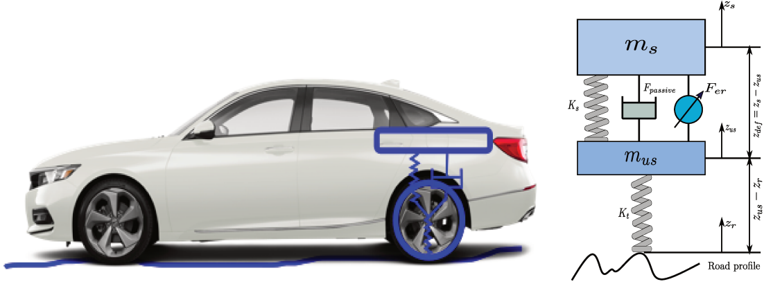
Figure 2.2: Quarter vehicle model
