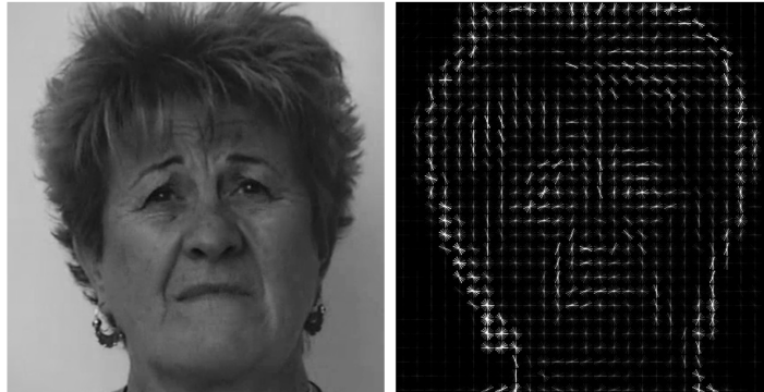
Figure 3.8: The raw input image corresponds to a frightened spontaneous expression class along its corresponding HOG features that encode gradient orientations.
