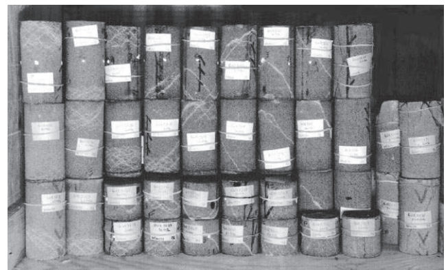
Fig. 7. Sandstone specimens tested in compression, at low (right) to high (left) values of the confining pressure.
