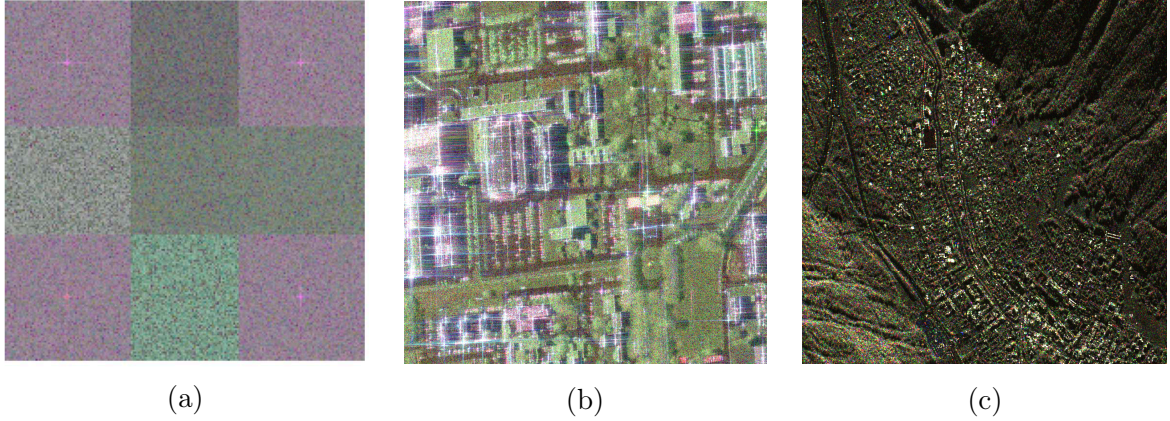
Figure II.1: Data sets: (a) Synthetic POLSAR data, intensity color composition of the target vector elements k_1-k_3-k_2 in Pauli basis, (b) Toulouse, RAMSES POLSAR data, intensity color composition of the target vector elements k_1-k_3-k_2 in Pauli basis, (c) TerraSAR-X 3-pass InSAR data, amplitude color composition of the complex random vector elements k_1-k_2-k_3 .
