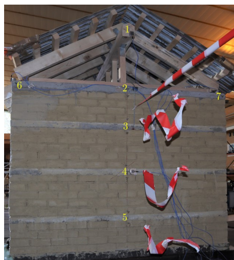
Figure 19. Positions of the cable sensors on the north wall of the reduced scale house.
