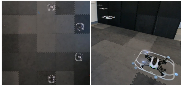
Fig. 1. Four mini UAVs forming two evenly spaced configurations: circular sector formation (left) and linear formation (right). Video of the real world experiments available at: https://youtu.be/wTe1MbYiZxs
