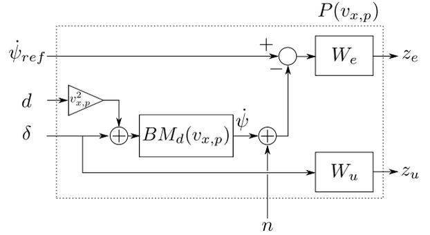
Figure 9: Generalized Plant Scheme at grid-point  $v_{x,p}$ .
