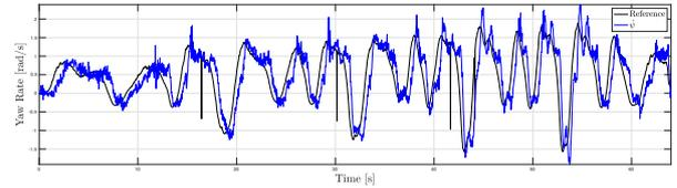
Figure 13: Yaw rate reference (black) and SAV yaw rate (blue) during the test.
