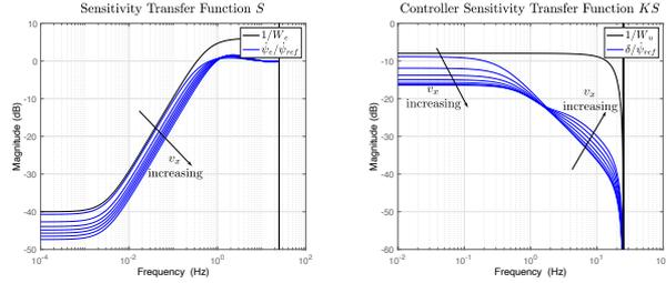
Figure 11: Sensitivity Transfer Function  $S = \frac{\dot{\psi}_e}{\dot{\psi}_{ref}}$  versus tracking performance template  $W_e^{-1}$  (left) and Controller Sensitivity Transfer Function  $KS = \frac{\delta}{\dot{\psi}_{ref}}$  versus actuator performance template  $W_u^{-1}$  (right) at frozen values of the varying parameter  $v_x$ .
