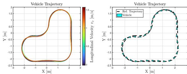
Figure 15: Reference trajectory and actual vehicle trajectory color coded with the instantaneous longitudinal velocity (left). Reference Trajectory and position and orientation of the SAV during a lap done at high speed at  $t \in [40, 50]sec$  (right).
