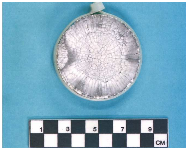
Fig. 10 Coarse-grained alumina disc recovered after a preliminary spherical expansion shock wave pyrotechnic test
