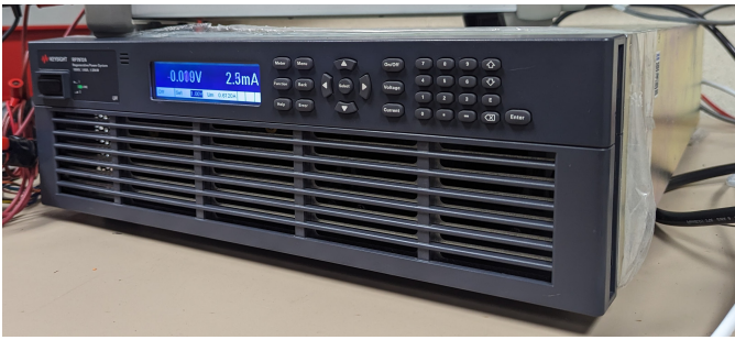
Fig. 3. The RP7972A Regenerative Power System provided by the ElectroMobility Laboratory at Tecnológico de Monterrey, a National Research Laboratory on ElectroMobility and autonomous vehicles.
