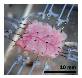
Figure 4. A biaxial tensile test experimental setup used to investigate the small intestine of pigs. Deformation is applied to a square sample ( $10 \text{ mm} \times 10 \text{ mm}$ ) through hooks attached to each side. Four graphite markers were placed on the surface of the sample to optically track its displacement during testing [74].
