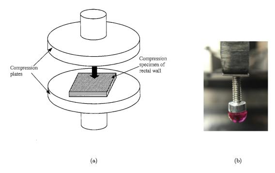
Figure 7. a) Schematic diagram of a uniaxial compression test being conducted on the rectum from pigs. The arrow indicates the direction the top plate moves during testing [79]. b) Semi-spherical indenter used to investigate the large intestine from rats. The indenter is rigid and has a 3 mm-diameter which comes into contact with the tissue during testing. Figure (b) modified from [80].
