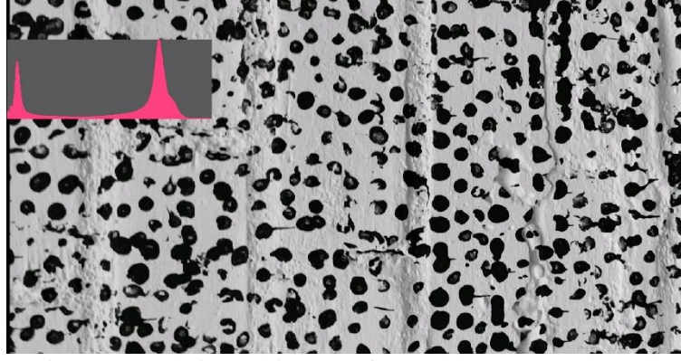
Fig. 8 Grayscale image histogram for speckle pattern on the wall surface
