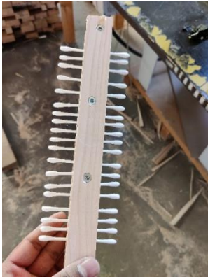
Fig. 7 Arrangement of cotton bud for application of black speckles pattern
