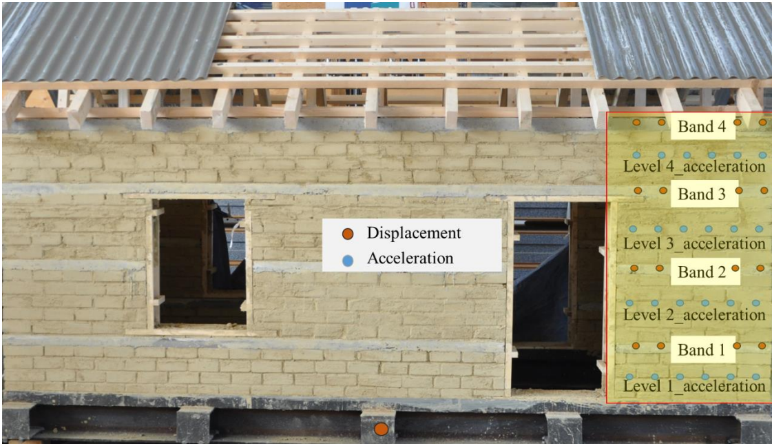
Fig. 18. Region selected for energy dissipation with a location represented for displacement and acceleration points
