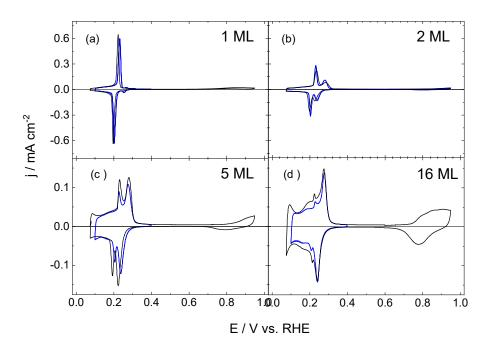
Figure S1. Cyclic voltammograms for  $Pd_{xML}/Pt(111)$  with (a) x = 1, (b) x = 2, (c) x = 5, (d) x = 16 in  $H_2SO_4$  0.1 mol  $L^{-1}$ , before (black line) and after (blue line) formic acid electrooxidation experiments.
