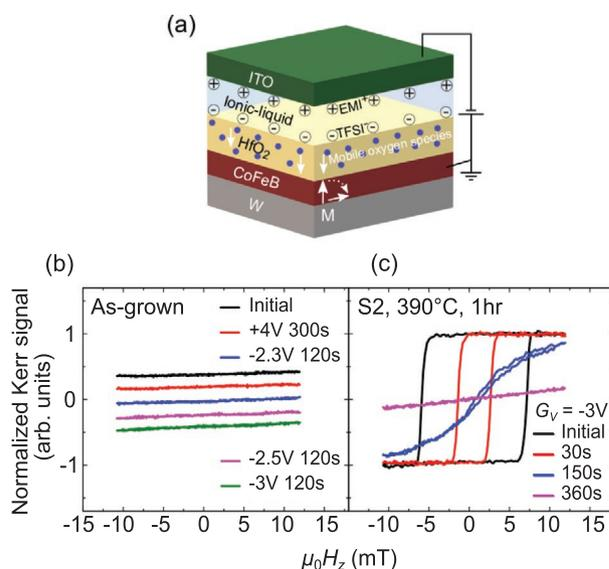
**Figure 1.** a) Schematic of the structure of the ionic-liquid gate device and pMOKE signal under an out-of-plane magnetic field ( $\mu_0 H_z$ ) of the b) as-grown, and c) annealed S2 sample under different gate voltages and gating times.
