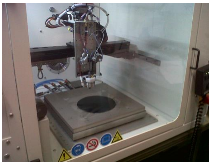
4380 Figure 109. Photograph of a catalytic ink printer used to spray catalytic inks onto PFSA membranes (batch process, lab-scale). Reproduced with permission from Paris-Saclay University.
