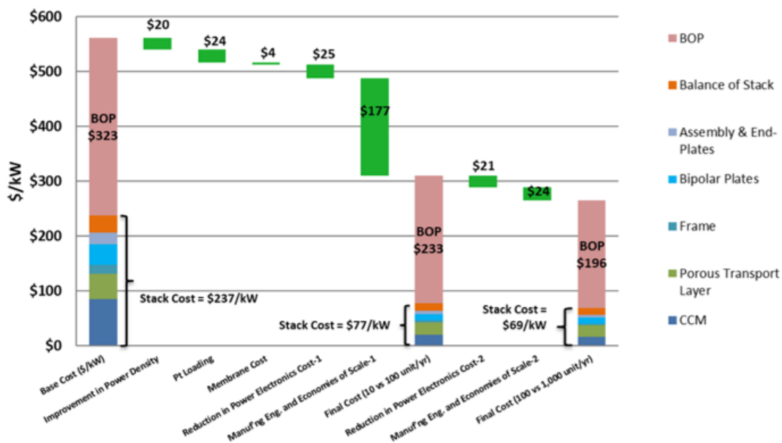
Figure 169. Future cost reductions for PEMWE systems across different production scales. Reproduced from Mayyas and Mann 1909 .
