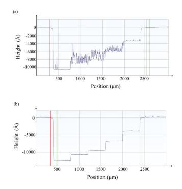
FIG. 6. The etched profiles of the stepcase shape transferred into Si (a): using Cl<sub>2</sub>, O<sub>2</sub>, HBr, (b): replacing the O<sub>2</sub> by He/O<sub>2</sub> with a power of 100 Wbias and 10 mTorr pressure.
