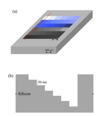
FIG. 1. (a) Illustration of a 2D micro-interferometers array of 960\*960µm<sup>2</sup> prepared in a silicon substrate, (b): cross section along the red line showing the targeted typical step height.
