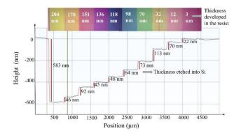
FIG. 9. Heights (in nm) and optical microscopy image of 10 strips patterned in the resist and the corresponding profile obtained by etching those resist patterns into silicon.
