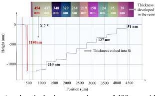
FIG. 5. Heights (in nm) and optical microscopy image of 400  $\mu$ m wide strips patterned in the resist with various power exposure ratios and the corresponding profile obtained by etching those resist patterns into silicon.
