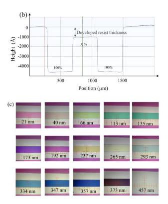
FIG. 4. (a): color code design of three strips, (b) the profile obtained in the resist, (c) heights (in nm) and optical microscopy image of strips ( $400*4000 \mu m$  per strip) patterned in the resist with various power exposure ratios.
