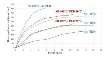
FIG. 7. Improvement of the contrast curve using various SB and PEB conditions in a 460 nm thick film of diluted ma-P1225G.
