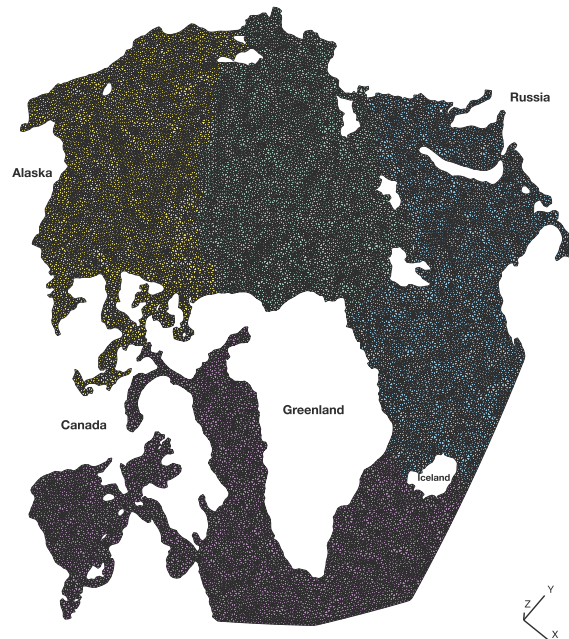
Fig. 5.1. Example of computational mesh at 30 km resolution covering roughly the same domain as used for our numerical experiments. The colours correspond to the 4 subdomains obtained after a mesh partitioning processed by METIS.
