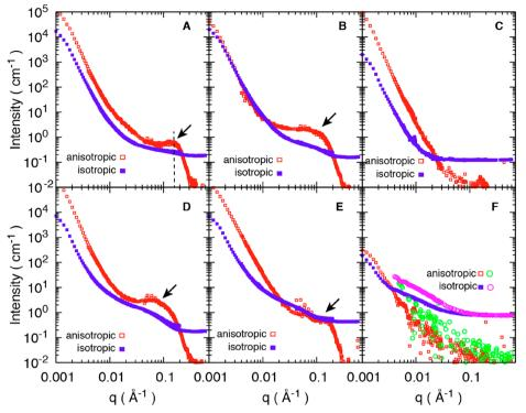
**Figure 3.** Decomposed anisotropic and isotropic SANS profiles from materials listed in Table 1: NatW/D<sub>2</sub>O (A), DelW/D<sub>2</sub>O (B), dry DelW (C), DelW/D-PMMA (D), DelW/PMMA (E), and DelW in liquid partD-MMA mixture (F, squares), and DelW/partD-PMMA (F, circles). Note that two materials are presented in (F). Arrows in the figures indicate the shoulder or peaks present in the high q region.
