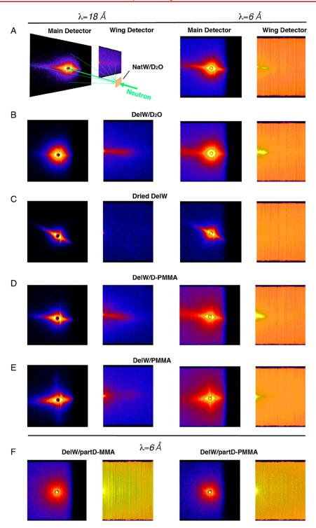
Figure 2. Two-dimensional SANS patterns at two incident neutron wavelengths. (A) NatW/D<sub>2</sub>O; (B) DelW/D<sub>2</sub>O; (C) dry DelW; (D) DelW/D-PMMA; (E) DelW/PMMA; (F) DelW/partD-MMA and DelW/partD-PMMA. Material designations are explained in Table 1.
