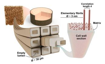
Figure 1. Cellular structure in wood, showing nine wood fibers and an enlarged view of a section of the cell wall nanostructure. Elementary cellulose fibrils are distributed in a "matrix", and the interfibril correlation length d between fibril centers is estimated using smallangle neutron and X-ray scattering (SANS/SAXS). Different samples have different compositions of the "matrix", see Table 1.
