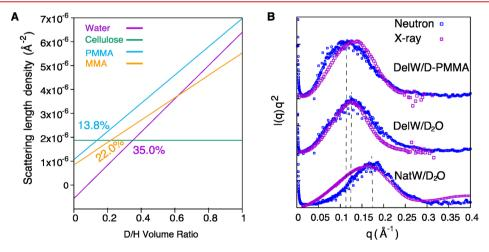
**Figure 4.** Neutron scattering length density of cellulose, water, PMMA, and MMA as a function of deuterium/hydrogen D/H ratio (A). The  $I(q)q^2$  profiles from SANS and SAXS for NatW/D<sub>2</sub>O, DelW/D<sub>2</sub>O, and DelW/D-PMMA (B).
