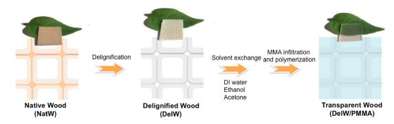
"NatW was Processed by Delignication, Solvent Exchange, MMA Monomer Infiltration Followed by Polymerization to Form Transparent Wood in the Form of DelW/PMMA.
