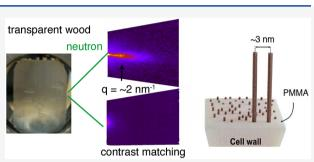
when contrast-matched PMMA is used, indeed proving nanoscale polymer distribution in the cell wall. The specific processing method used for transparent wood explains the nanocomposite nature of the wood cell wall and can serve as a nanotechnology for cell wall impregnation of polymers in large wood biocomposite structures.
