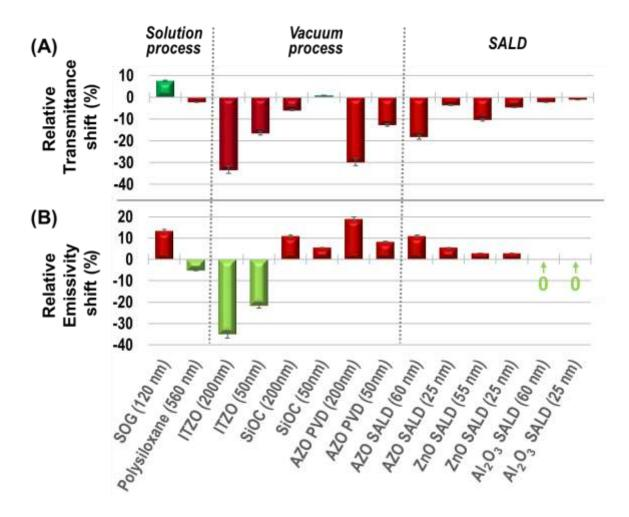
**Figure 3.** Protective layer impact on low-E coating optical properties: (a) Relative transmittance (measured at 550 nm) shift and (b) relative emissivity shift (2-20  $\mu$ m) induced by deposition of different protective layers on AgNWs networks, when compared to the non-coated AgNW network.
