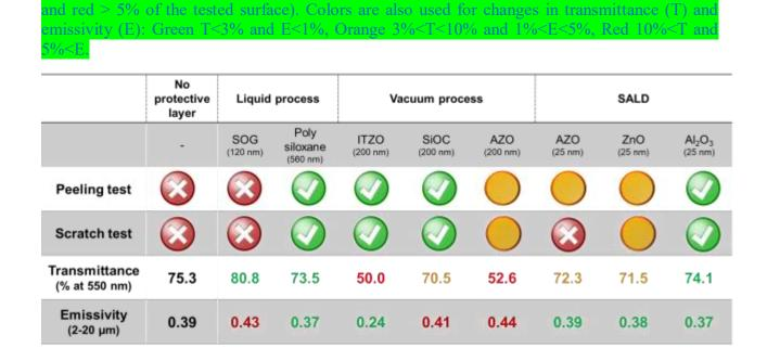
**Table 1.** Compilation of the optical and mechanical results of the encapsulated AgNWs based
