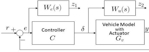
Fig. 3. Lateral control design via yaw-rate tracking.
