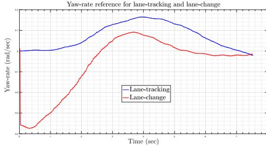
Fig. 1. Yaw-rate references for the case of tracking a turn (blue) and for a lane-change maneuver (red) recovered in experimental tests while driving in autonomous mode an automated Renault Zoe for  $v_x = 10m/s$ .
