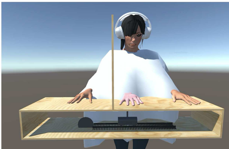
Figure 1. Experimental set-up. The participant sat in front of a table, facing his left hand and the rubber hand. Participants wore a hairdresser's blouse to ensure that no gap were visible between the participants' body and the rubber hand. An opaque board occluded the right hand from his view. The motorized train positioned under the table could move the rubber hand in the lateral (as shown here) or the sagittal axis, according to the Experiment. The hidden right hand (but also the left one) was always static.
