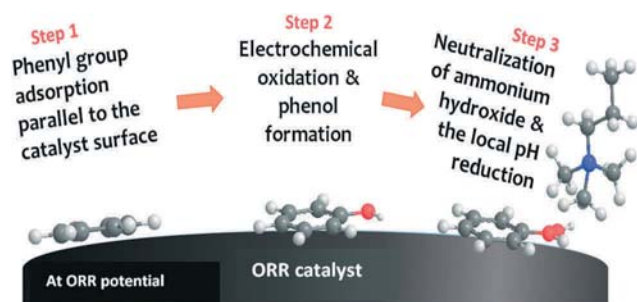
Fig. 7 Quaternary ammonium neutralization process by electrochemical phenyl oxidation at ORR potential. The scheme is reproduced from ref. 208.
