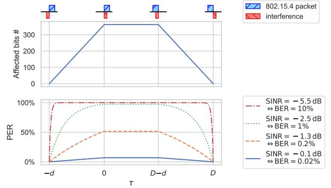
Fig. 3. Interference between an IEEE 802.15.4 frame of duration  $D = 4.10$  ms and interference of duration  $d = 1.45$  ms.  $\tau$  is the difference (in time) between the beginning of the frame and the interference. The impact of the interference is longer than their respective durations and a high interference level quickly results in almost 100 % PER during the whole timespan.
