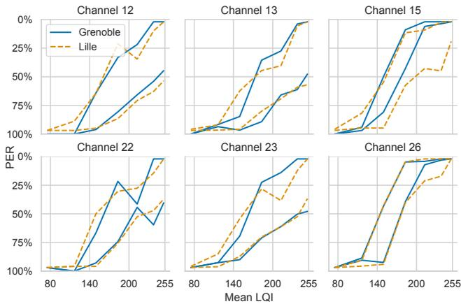
Fig. 1. Quantile regression (5<sup>th</sup> and 95<sup>th</sup> percentile) of PER with respect to LQI.
