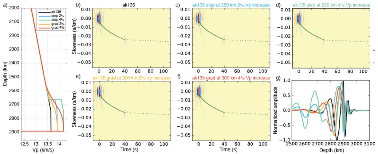
Figure 7: (a) proposed velocity models. (b-f) Vespagrams computed for each model at a distance of  $62^\circ$ . (g)  $I_z$  functions obtained following the same process as in Figure 6b and for each model.
