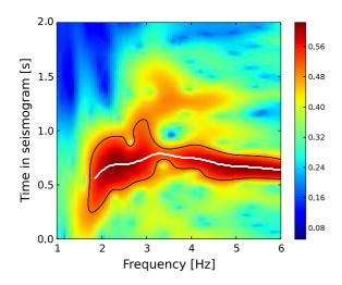
Figure 4 Rayleigh wave group velocity dispersion curve in the time-frequency domain for two stations located at x=-289 m and x=124 m. The colors indicate amplitude after logarithmic stacking of negative-lag and positive-lag ZZ, ZR, RZ, and RR correlation waveforms. The black contour indicates the 0.5 threshold described in the text. The white section of the peak-amplitude line indicates data used in the analysis. The  $1\lambda$  distance threshold applies below 1.8 Hz
