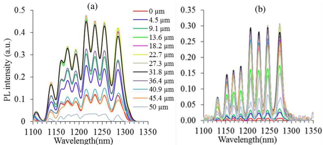
Figure 6. Series of  $\mu$ PL spectra measured at low temperature (10 K) across 50  $\mu\text{m}$  ridges. (a) etching with  $\text{CH}_4/\text{H}_2/\text{Ar}$ , and (b) etching with  $\text{Cl}_2/\text{CH}_4/\text{Ar}$ . Each color corresponds to a different position across the ridge as indicated by the legend in the center. The center of the ridge corresponds to the 25  $\mu\text{m}$  position.
