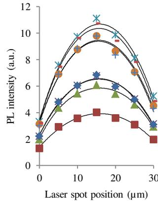
Figure 12. Curve fitting and experimental QW line intensities across a 30 μm stripe with etch depth 2 μm after the CH<sub>4</sub>/H<sub>2</sub>/Ar process. The symbols have the same meaning as in figure 7.
