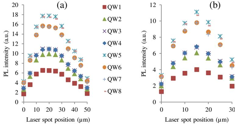
Figure 7. Integrated intensity for individual PL lines across stripes with etch depth  $2\ \mu\text{m}$  after the  $\text{CH}_4/\text{H}_2/\text{Ar}$  process. (a) Stripe width  $50\ \mu\text{m}$ , and (b) stripe width  $30\ \mu\text{m}$ .
