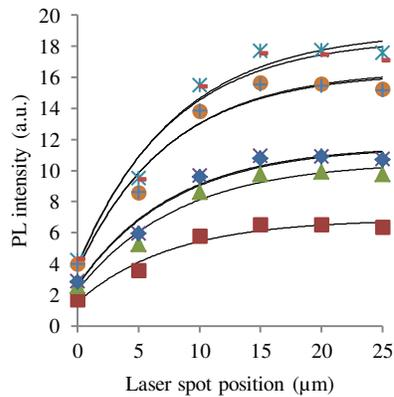
Figure 13. Curve fitting and experimental QW line intensities across a 50  $\mu\text{m}$  stripe (left edge) with etch depth 2  $\mu\text{m}$  after the  $\text{CH}_4/\text{H}_2/\text{Ar}$  process. The symbols have the same meaning as in figure 7.
