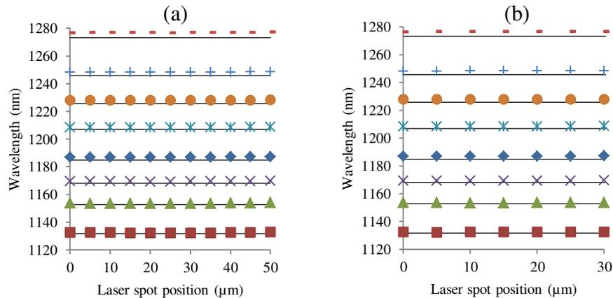
Figure 11. Spectral positions for individual PL lines across stripes with etch depth 2  $\mu\text{m}$  after the  $\text{CH}_4/\text{H}_2/\text{Ar}$  process. The straight lines represent the corresponding positions on the reference, un-etched, sample. (a) Stripe width 50  $\mu\text{m}$ , and (b) stripe width 30  $\mu\text{m}$ .
