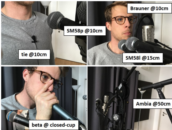
Figure 2: Placement of all microphones : tie, Braun, SM58 at 10cm and 15 cm, ambient at 50 cm, and Beta SM58 with closed-cup technique
