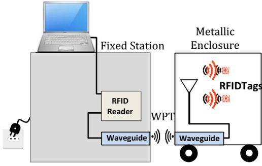
Fig. 1. Reading RFID tag with WPT system
