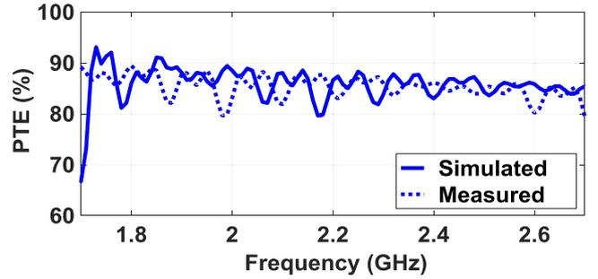
Fig. 7 PTE of the rectangular waveguide WR 430
