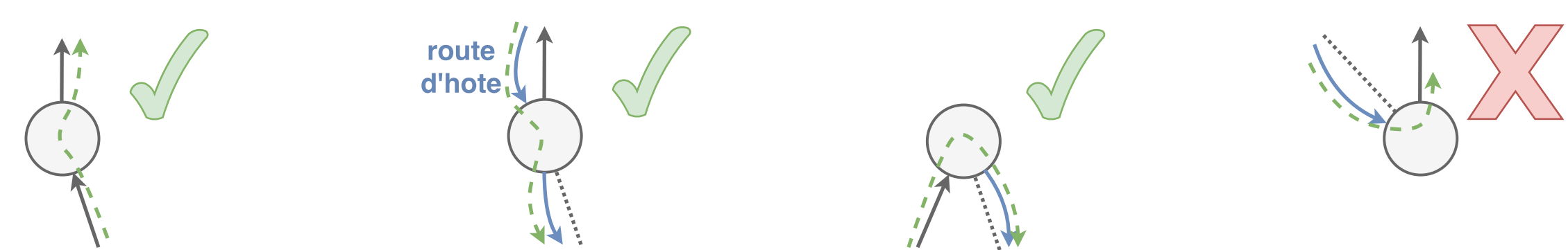
Figure 4: Routing loop detection. In the last case, the node should use a route which is less precise than the previous one, that is forbidden.
