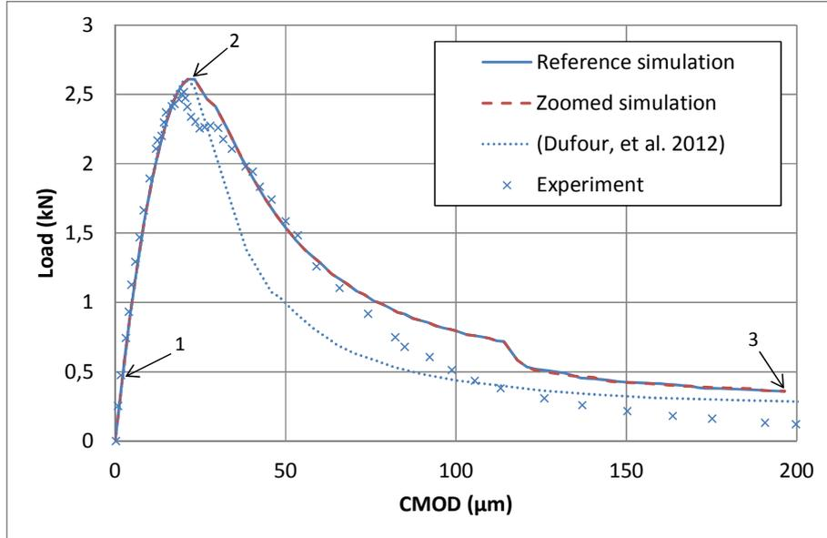
Figure 5: Comparison of load-CMOD evolutions of the reference and zoomed simulation.
