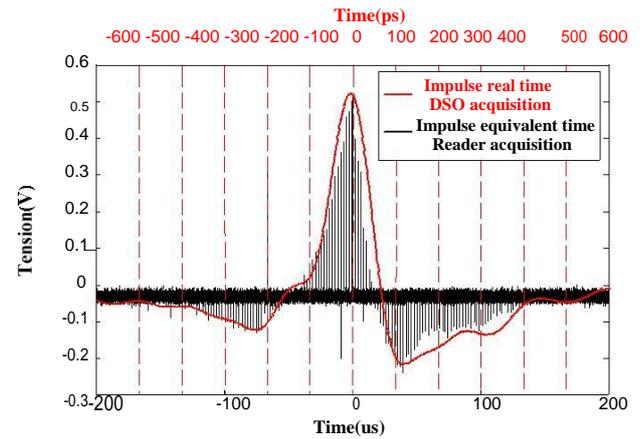
Fig. 4. Comparison between the attenuated output of the pulse generator, measured with a DSO, and the input of the ADC of the second reader in order to appreciate the sampling noise of the system and the equivalent time algorithm.
