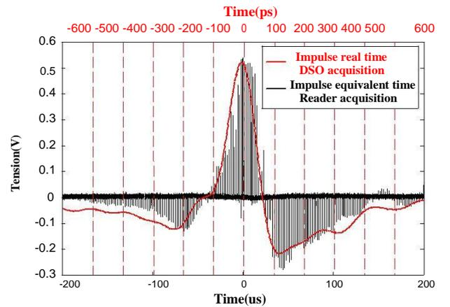
Fig. 2. Comparison between the attenuated output of the pulse generator, measured with a DSO, and the input of the ADC of the first reader in order to appreciate the sampling noise of the system and the equivalent time algorithm.
