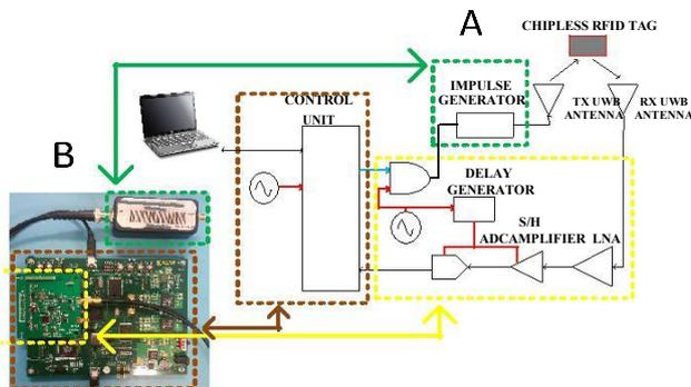
Fig. 3. Block diagram(A) and photo(B) of the second realized reader for chipless RFID tags. The control unit is entrusted on a FPGA Xilinx spartan 6 on the evaluation board SP601. The RF part is the smallest PCB on top of the SP601. The RF PCB presents a second clock generator and an ultra-low jitter AND gate to decrease the sampling noise of the system.
