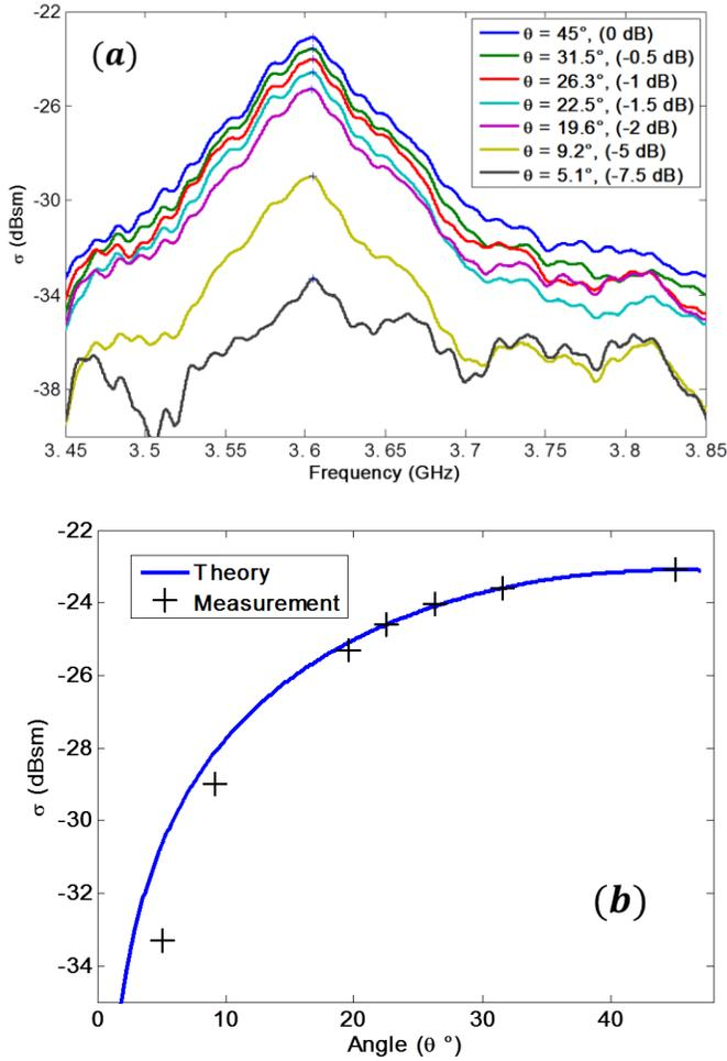
Fig. 4. (a) Measurement of the RCS magnitude of the peak  $n=2$  of the tag of Fig. 2 for different values of angle  $\theta$ . (b) Comparison between the measured and the calculated magnitude using (4).
