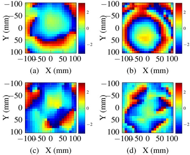
**Figure 4.** Phase variation as a function of the position on the plan, (a) for the first resonant frequency (3.19 GHz), (b) for the 8th resonant frequency (6.78 GHz), (c) between first and second peak (3.39 GHz), (d) after the 8th peak (7.70 GHz).
