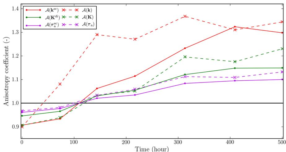
**Figure 12.** Time evolution of the anisotropy coefficients of air tortuosity, thermal conductivity and permeability. Comparison between coefficients deduced from values computed on 3-D images (dashed lines) and values given by analytical estimates (solid lines).
