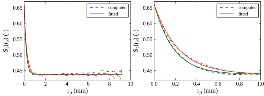
**Figure 3.** Two-point probability function  $S_2(\mathbf{r})$  for the whole range of  $\mathbf{r}$  (left panel) and magnified (right panel) in the  $x$  (blue),  $y$  (green) and  $z$  directions (red), obtained from the 3-D image referred to as 7G in Table 1. Solid and dashed lines correspond, respectively, to the values computed from Eq. (3) and to the results of the expression  $S_2(r_\beta) = (\phi - \phi^2) \exp(-r_\beta/l_{c_\beta}) + \phi^2$  with  $\beta = (x, y, z)$ .
