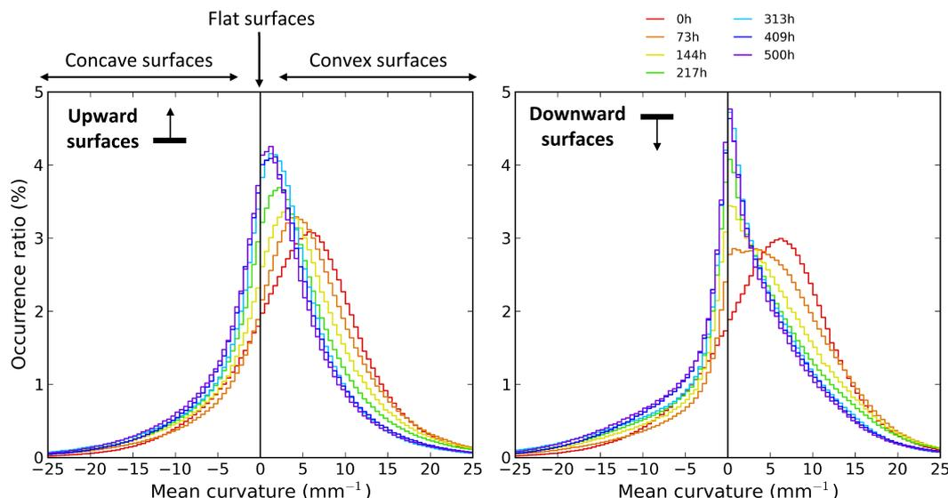
**Figure 8.** Time evolution of the mean curvature distribution computed from the upward (left panel) and downward (right panel) surfaces of the 3-D images. Each curvature class is  $0.5 \text{ mm}^{-1}$  wide.
