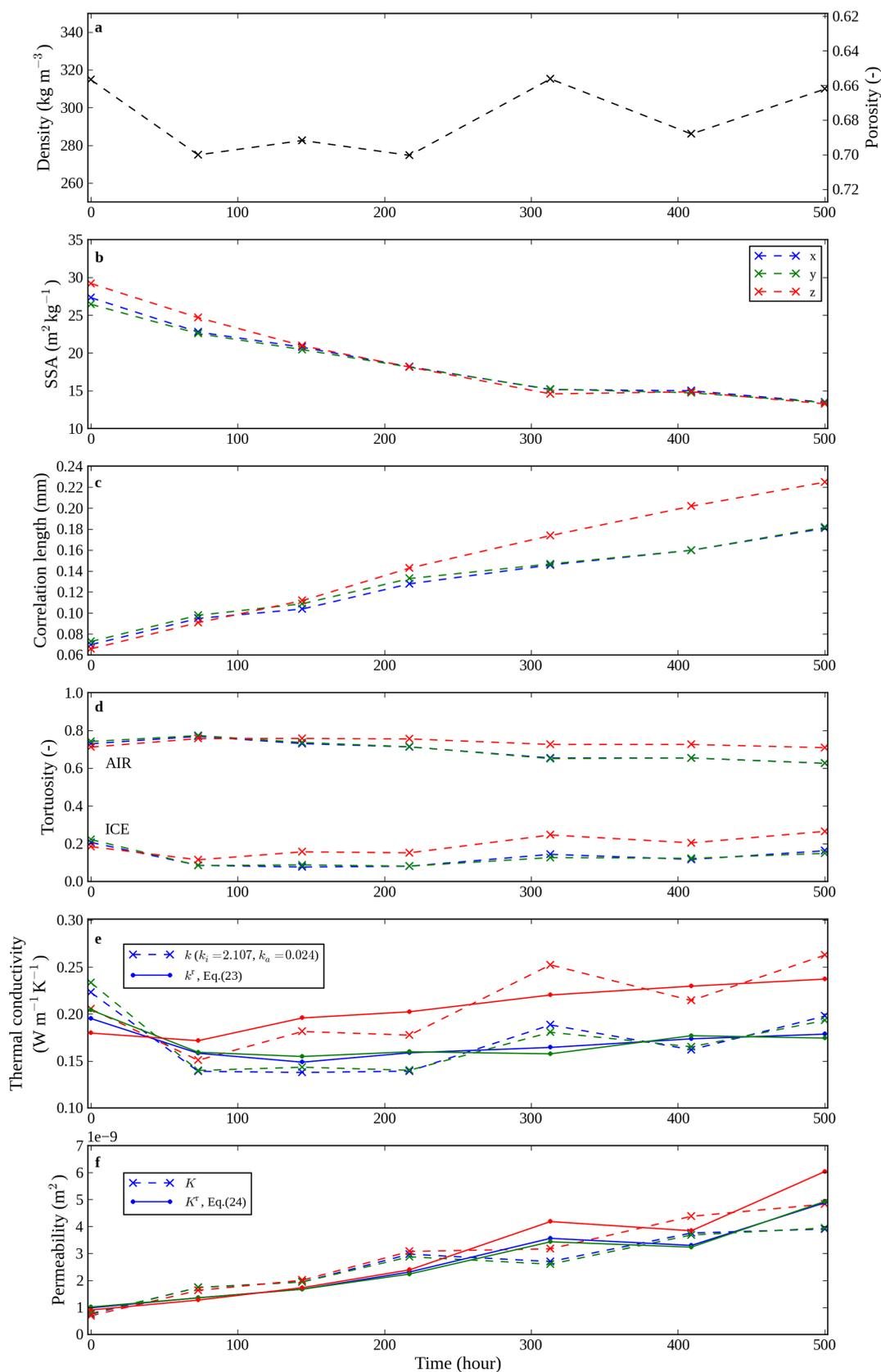
**Figure 6.** Time evolution of microstructural and physical properties of snow during the whole temperature gradient experiment. Values in the  $x$ ,  $y$  and  $z$  directions are given in blue, green and red, respectively.
