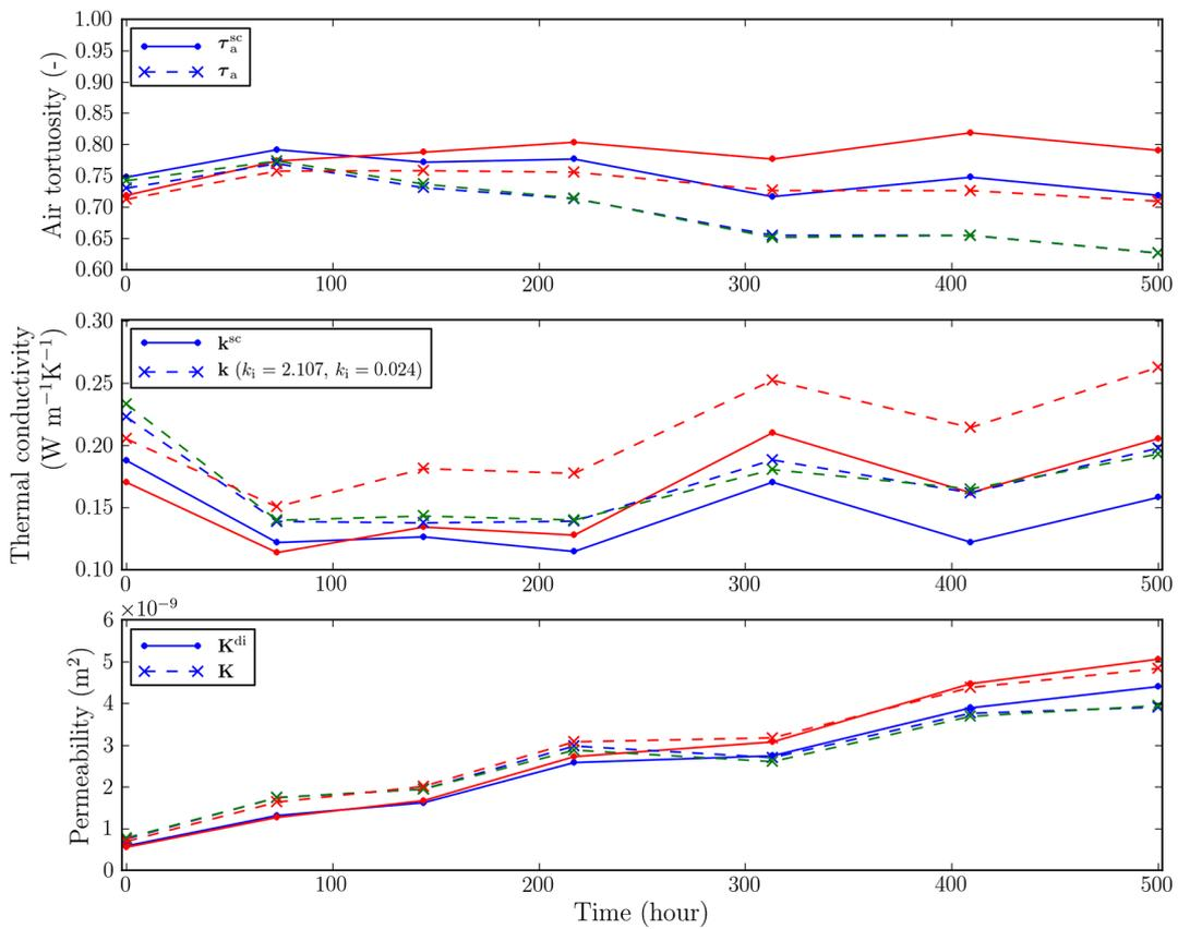
**Figure 11.** Time evolution of air tortuosity, thermal conductivity and permeability during the whole experiment. Comparison between values computed from 3-D images in the  $x$ ,  $y$  and  $z$  directions (dashed lines in blue, green and red, respectively) and values given by analytical estimates in the  $x$   $y$  and  $z$  directions (solid lines in blue and red, respectively).
