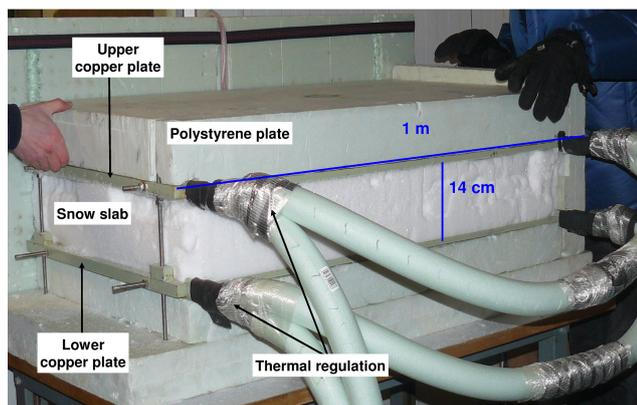
**Figure 1.** Photograph in cold room of the apparatus designed to control and monitor temperatures at the top and bottom of a snow slab. The front and side vertical polystyrene plates were removed from the device for visualization purposes.
