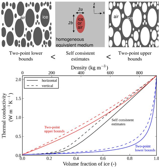
**Figure 4.** Schematic representation of the microstructure corresponding to the two-point bounds and the self-consistent scheme. Effective thermal conductivity versus ice volume fraction when  $b/a = 1.45$ : self-consistent estimates (black curves), two-point lower (blue curves) and upper (red curves) bounds.
