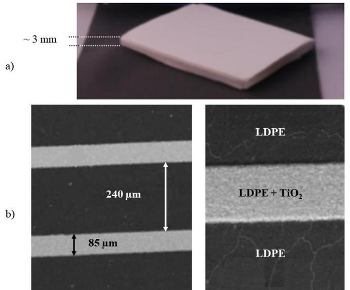
Fig.1 a) Picture of the experimental sample multilayer tag;
