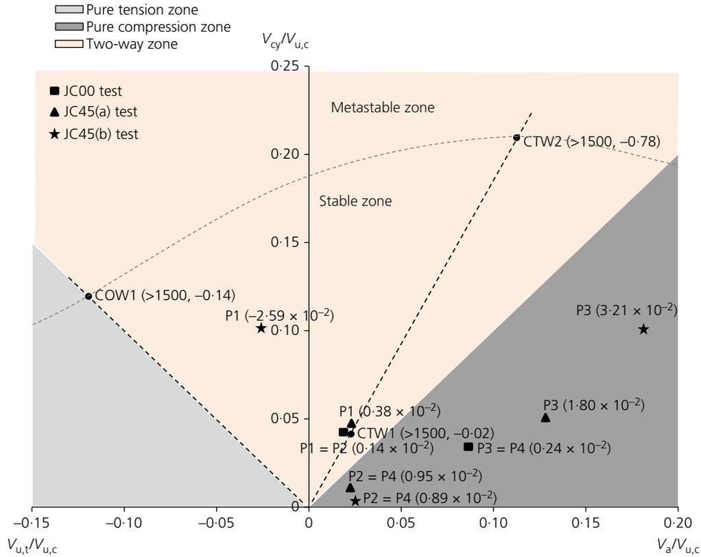
**Figure 10.** Stable zone of the stability diagram for single and jacket piles (prototype scale)
