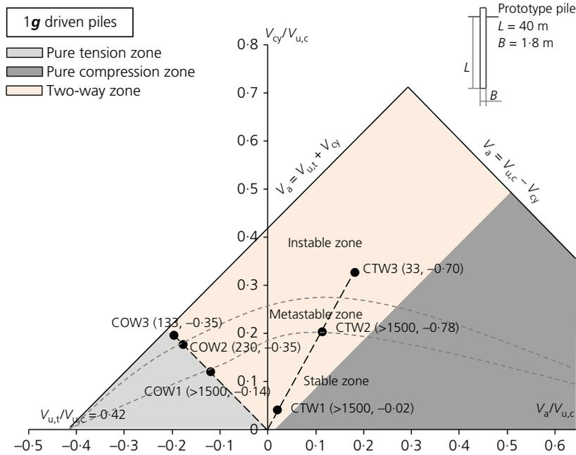
Figure 9. Stability diagram of 1g jacked piles tested at 100g
