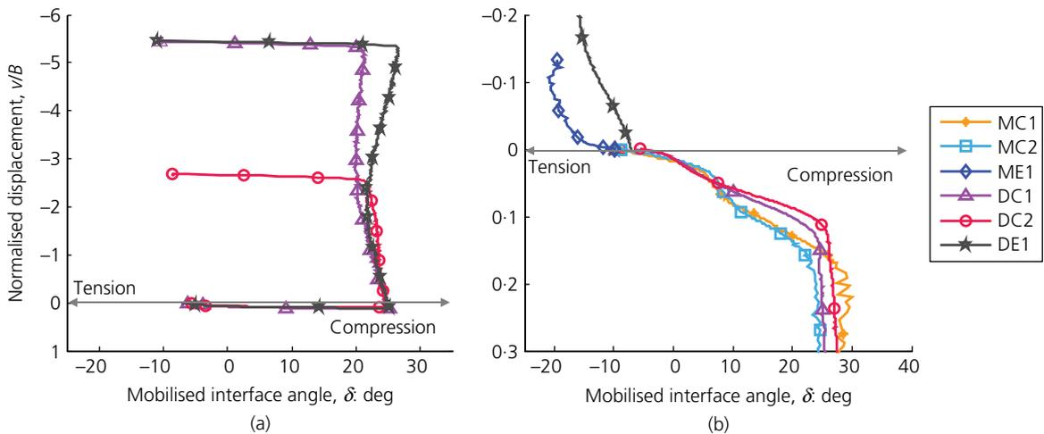
**Figure 7.** Monotonic loading test mobilised interface angle of friction (prototype scale): (a) jacking phase and (b) loading test
