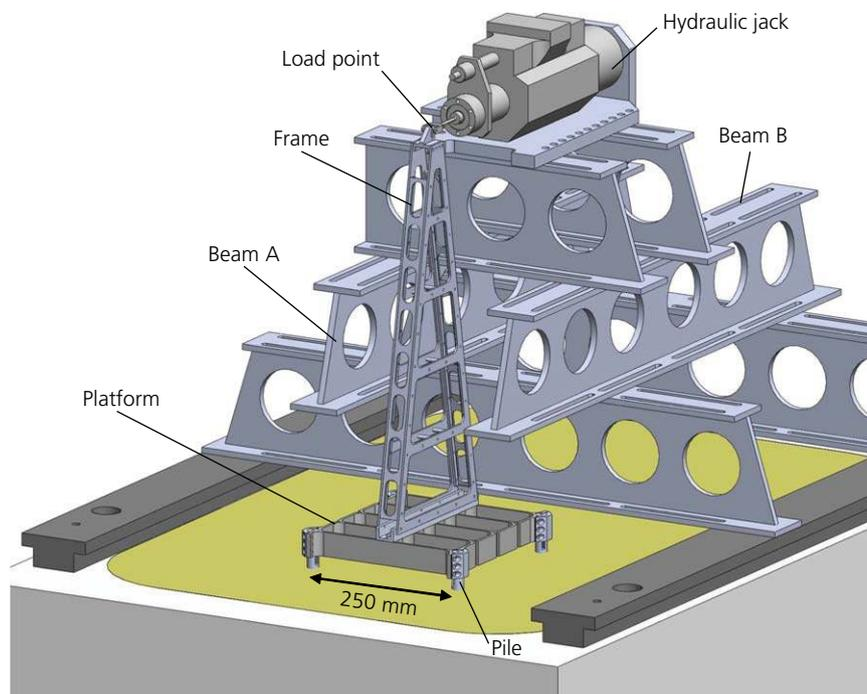
Figure 2. Centrifuge experimental set-up (0° jacket test)
