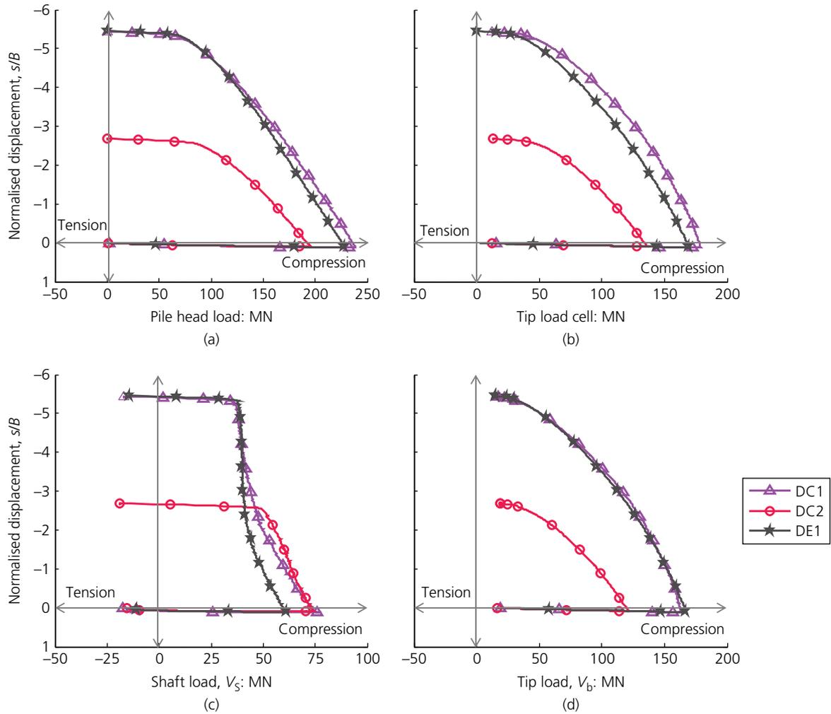
**Figure 5.** Jacking phase for monotonic loading tests (prototype scale): (a) load head sensor, (b) tip load cell, (c) shaft resistance against normalised displacement and (d) tip load against normalised displacement
