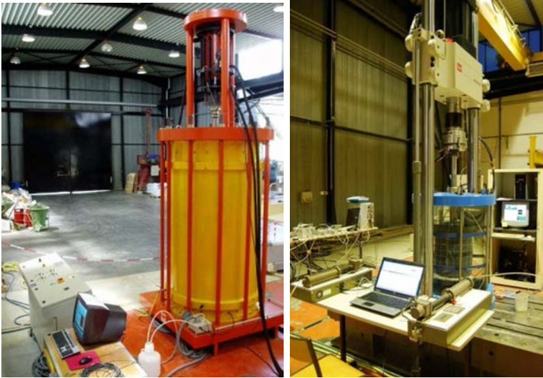
Figure 4.1. Large triaxial cells \Phi 1000 mm (left) and \Phi 250 mm (right). For a color version of the figure, see www.iste.co.uk/millet/advances.zip
