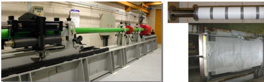
Figure 2. Gas launcher, deformable projectile and target.
