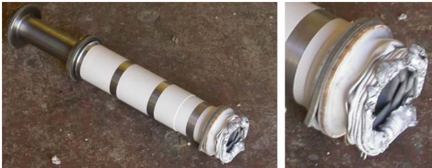
Figure 5. Deformation of the missile after perforation (test no. 2, V_0 = 70.2 m/s).
