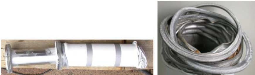
Figure 3. Deformation of the missile after perforation (test no. 1, V_0 = 107.5 m/s).
