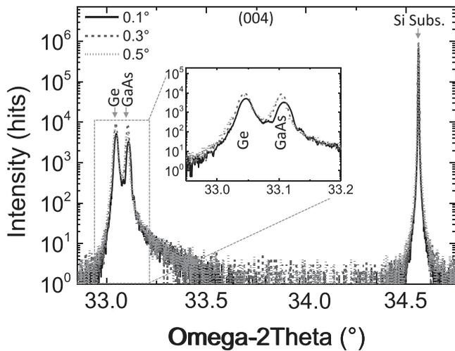
FIG. 1. High resolution, X-ray diffraction profiles around the (004) order (in the triple axis configuration) for a GaAs layer grown on a Ge-buffered silicon substrate with a  $0.1^\circ$  (solid line),  $0.3^\circ$  (dashed line), and  $0.5^\circ$  (dotted line) offcut.
