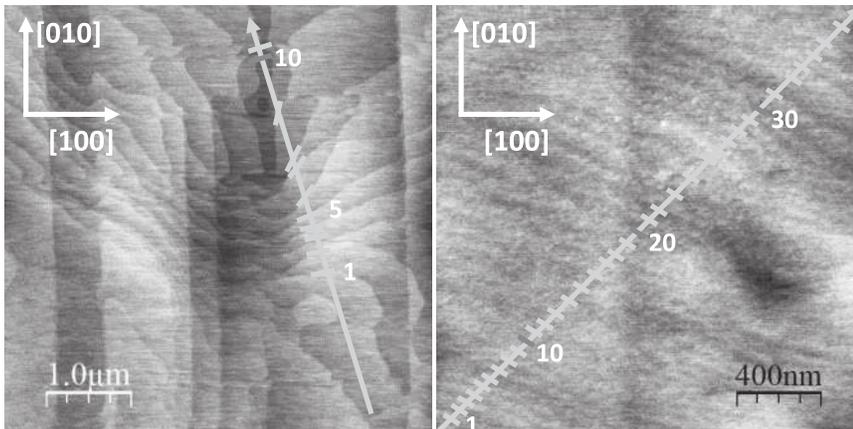
FIG. 4. Atomic Force Microscopy images of the Ge surface of samples grown on two different offcut angle silicon substrates. The left image corresponds to a  $0.04^\circ$  offcut (001) substrate, and the right image corresponds to a  $0.28^\circ$  offcut (001) substrate.
