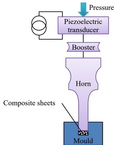
Figure 1: Schematic representation of the ultrasonic compression machine.
