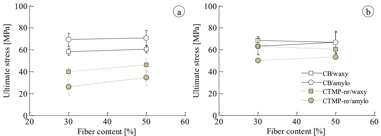
Figure 7: Ultimate strength of pulp/starch composites as a function of fibre content for (a) thermo-compression moulding, and (b) ultrasonic compression moulding.
