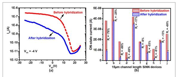
**Figure 6.** Electrical response of: (a) SiNN FET with L = 15  $\mu$ m before and after DNA hybridization, (b) ON-state current change of 10 devices with L = 15  $\mu$ m, the letter refers to the measured SiNN FETs.
