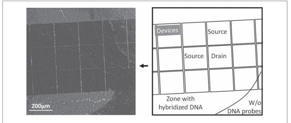
**Figure 5.** Florescence microscopy image of FETs after DNA hybridization using Cy3 labelled DNA targets with a sketch for better clarity (W/o = without).
