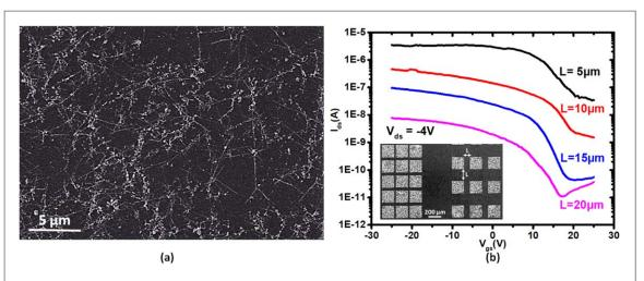
**Figure 3.** (a) SEM image of SiNW network elaborated from 28 ml of NW suspension and transferred onto Si/Si<sub>3</sub>N<sub>4</sub> substrate, (b) Transfer characteristics of FETs with L ranging from 5  $\mu$ m to 20  $\mu$ m.
