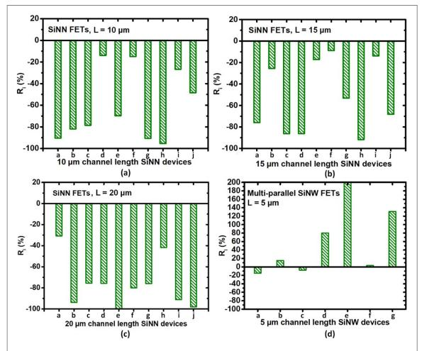
**Figure 7.** Relative variation of the ON-state current to DNA hybridization of: (a)  $L=10~\mu m$ ; (b)  $L=15~\mu m$ ; (c)  $L=20~\mu m$ ; (d)  $L=5~\mu m$ ; the letter refers to the measured FET.
