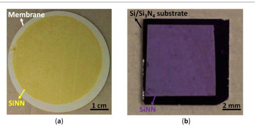
Figure 1. (a) Nanonet assembled on a nitrocellulose membrane, (b) Nanonet transferred onto 200-nm-thick  $\mathrm{Si}_3\mathrm{N}_4$  covered silicon substrate.
