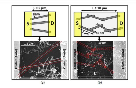
**Figure 2.** Two configurations of field effect transistors: (a) MP- SiNW FETs, (b) SiNN FETs. The nanowires have an average diameter of  $40\pm7$  nm and a mean length of  $7\pm3$   $\mu$ m; S= source, D= drain, the two electrodes of the FET; gate is on the back side.
