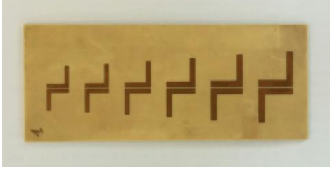
Figure 1. Chipless RFID tag used for gesture recognition.
