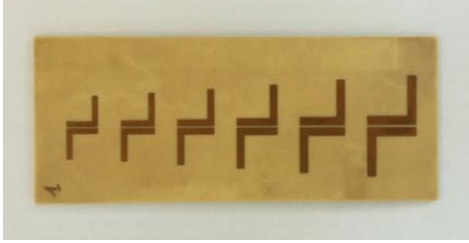
Figure 1. Chipless RFID tag used for gesture recognition.
