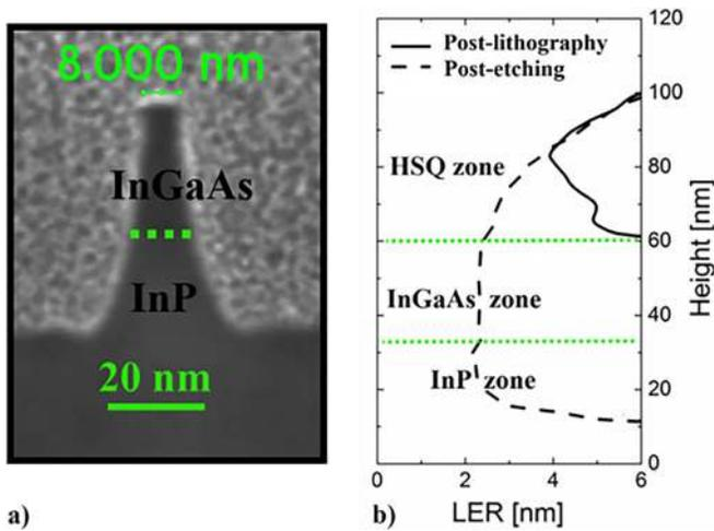
FIG. 6. (Color online) (a) FIB-STEM view of a 8 nm InGaAs fin realized using  $\text{BCl}_3/\text{SiCl}_4$  etch process (b) analysis by tilting AFM of the sidewall line edge roughness of the initial HSQ mask (dashed line) and the InGaAs/InP etched fins (continuous line).
