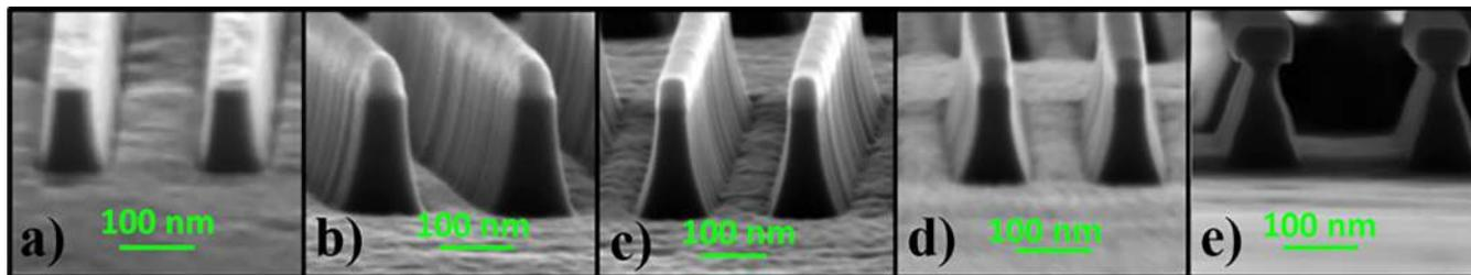
FIG. 5. (Color online) InGaAs fins obtained under different experimental conditions: (a) optimum process (ref.)  $\text{BCl}_3/\text{SiCl}_4/\text{Ar}$  flow ratio = 15/5/20 SCCM, (b) carrier wafer:  $\text{SiO}_2$  (vs Si), (c)  $\text{BCl}_3/\text{SiCl}_4/\text{Ar}$  flow ratio = 10/5/25 SCCM (vs 15/5/20 SCCM), (d) ICP power = 100 W (vs 50 W), and (e) RF platen power = 50 W (vs 150 W).
