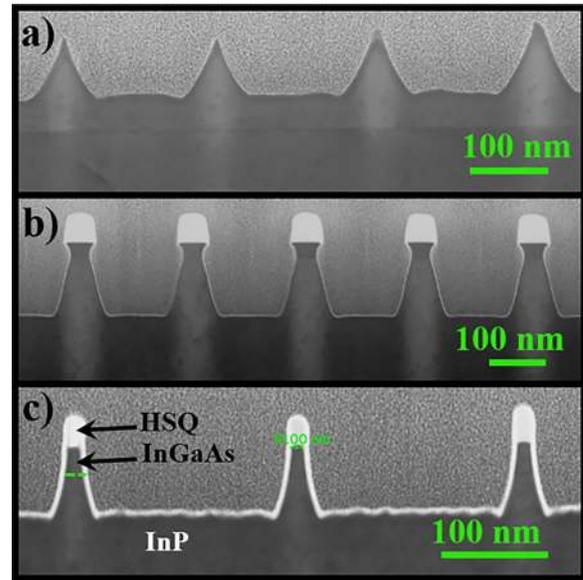
Fig. 3. (Color online) FIB-STEM images depicting the etching profiles of 10 nm wide fins obtained with three different chlorine plasma chemistries: (a)  $\text{Cl}_2/\text{Ar}$ , (b)  $\text{SiCl}_4/\text{Ar}$ , and (c)  $\text{BCl}_3/\text{Ar}$ .
