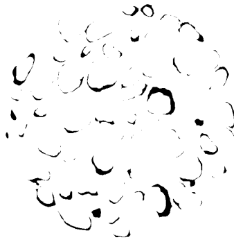
Figure 10: Characteristic slice of the difference between the two binarised 3D images (neutron and x-ray scan).
