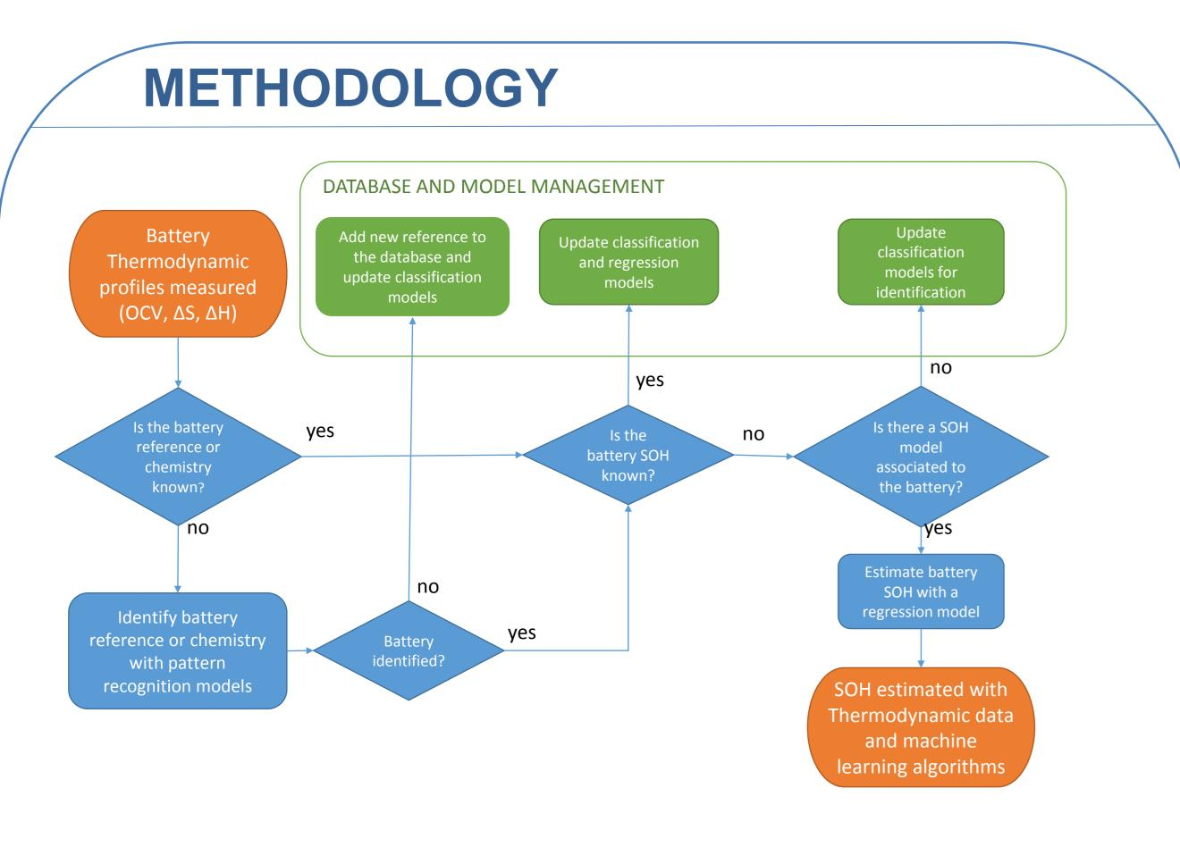
This diagram explains the process in order to estimate battery SOH from
