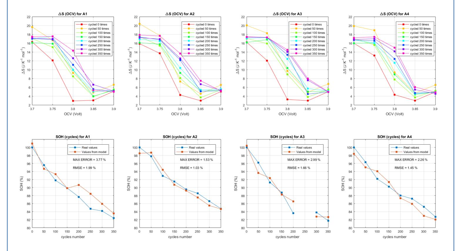
Graphs in the first row represent  $\Delta S$  data between 3.7 and 3.9 volts of the OCV at different ageing. Each graph of this row corresponds to a given battery.
