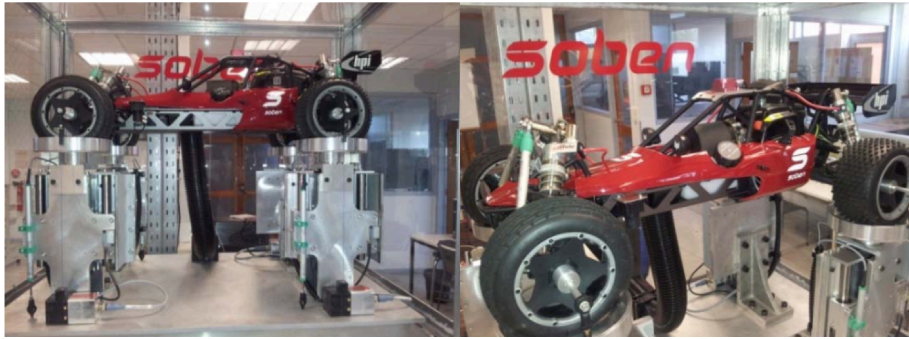
Figure 4: INOVE Soben-Car Test-Bench, see website [35]
