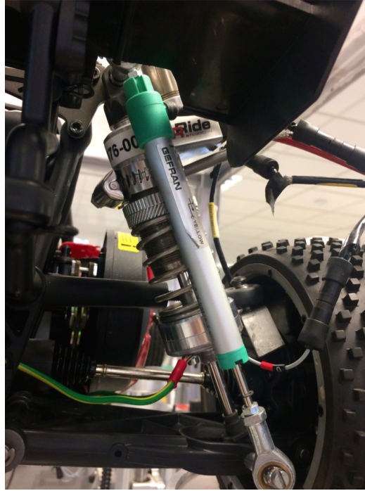
Figure 3: Electro-Rheological Damper on INOVE Soben-Car Test-Bench
