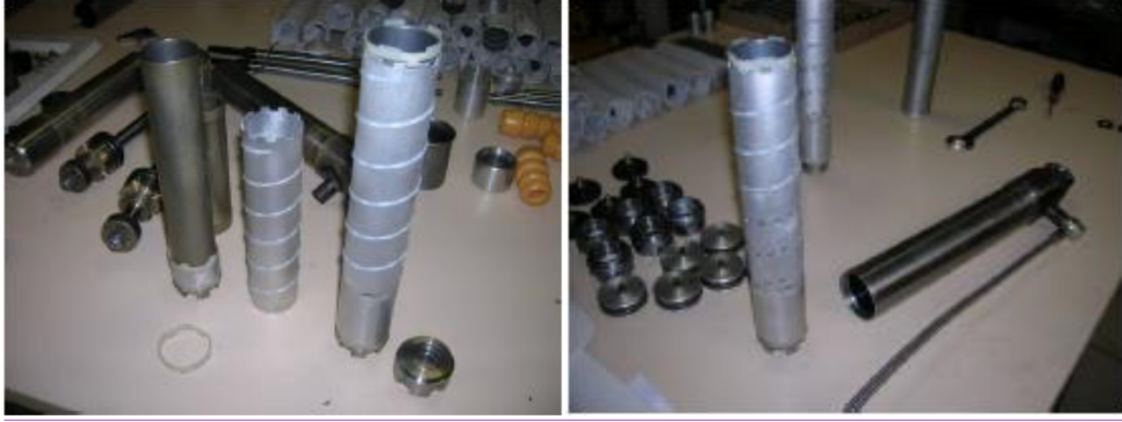
Figure 16: Spirals of the inner electrode of an ER Damper - Faultless (left) and Faulty (right)
